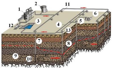
1, 2 - tanks for reagent and solutions, 3 - primary solution storage, 4 - piping of technological wells, 5 - well head, 6 - pump and compressor group, 7 - technological well, 8 - dynamic level of the solution in the formation, 9 - reservoir, 10 - well filter, 11 - injection wells, 12 - pump, 13 - pumping wells
