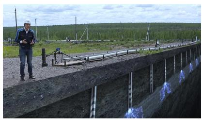
At the pilot block of Underground Leaching with a solution capacity of 15-25 m³/h, taking into account the hydrogeological conditions of the site, an infiltration-filtration system for borehole mining of the ore / formation massif with airlift elevation of productive solutions was developed and implemented. Coal sorption technology has been adopted to extract gold from solutions.
