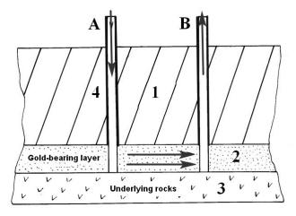
Initially, in the array 1, a bush of technological wells A and B is drilled, opening the formation 2 of compacted gold-bearing rocks to the underlying rocks 3. The wells are cased with pipes 4, equipped with heads, hydraulic fracturing between wells A and B of formation 2 and acidification are carried out. Then, efficient and environmentally friendly solutions of alkali and alkaline earth metal oxychloride are
